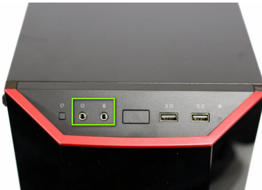
Pic 2 – Computer with headphone and microphone inputs. Note that the headphone symbol does not have a mic boom.
