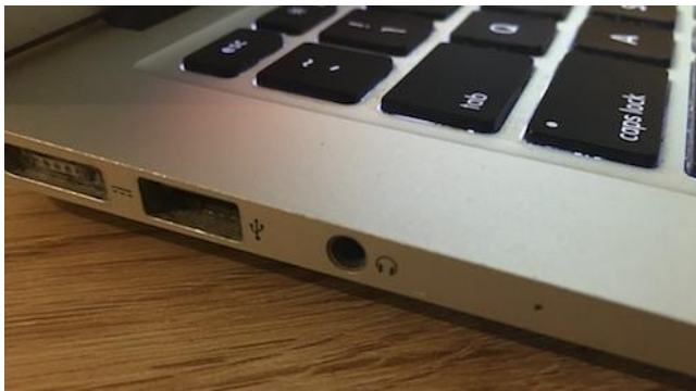
Pic 4 – Laptop with only a headphone plug (no microphone input). Note: no microphone boom on the headphone symbol.
