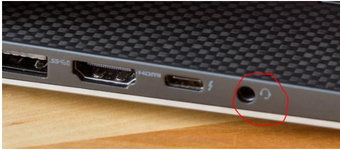
Pic 3 – Laptop with a headset (headphone and microphone combined) plug. Note the microphone boom in the headset symbol.
